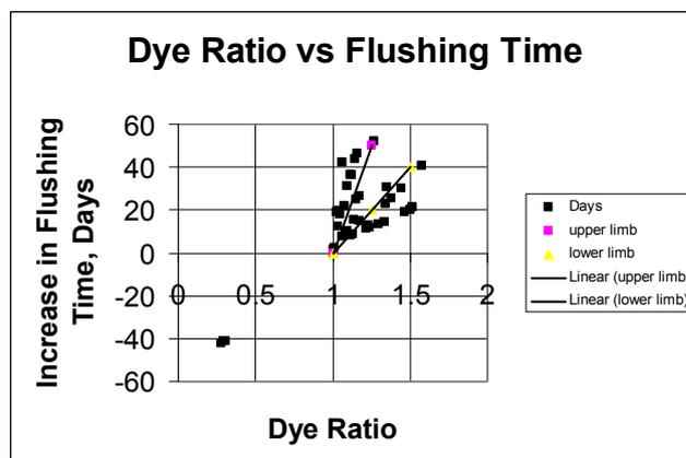
Figure 2. Relationships between  $C_{wd}/C_{nd}$  Ratio and Change in Flushing Time with Two Limbs
