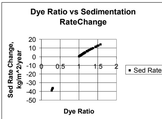
**Figure 7.** Relationships between  $C_{wd}/C_{nd}$  Ratio and Change in Settling Rate
