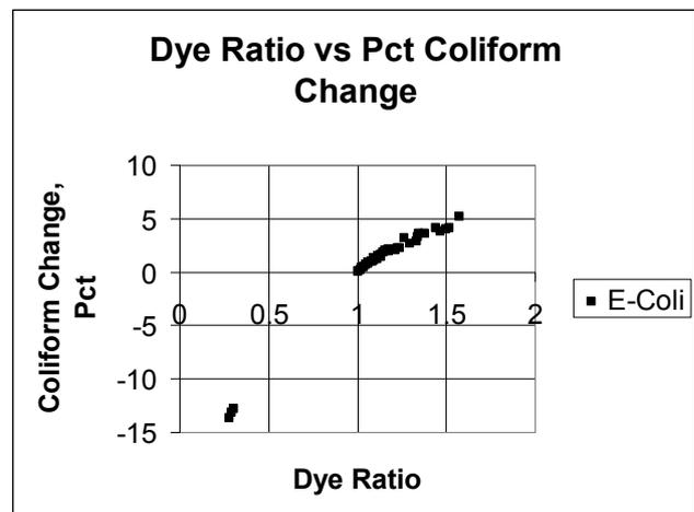
Figure 3. Relationships between  $C_{wd}/C_{nd}$  Ratio and Change in Coliforms
