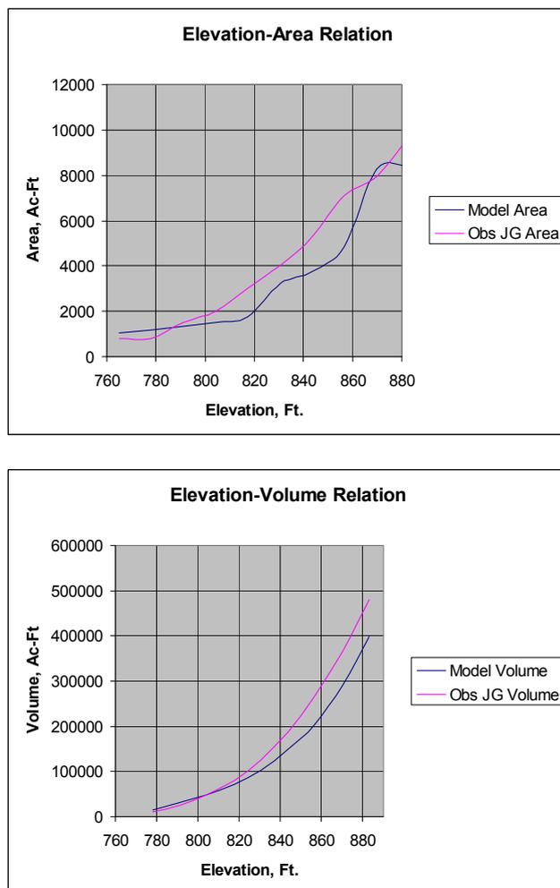
**Figure 1.** Comparison of Model Digital Bathymetric Hypsographs with TVA Data
