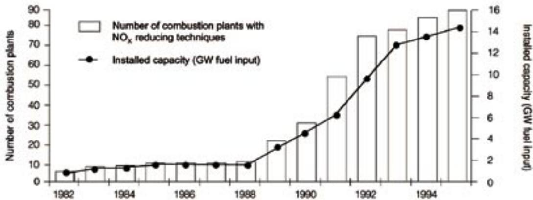
**Figure 4.** Installations of present and planned NO<sub>x</sub> reducing techniques during 1982 – 1994, (Source: IISD, 1994:25)
